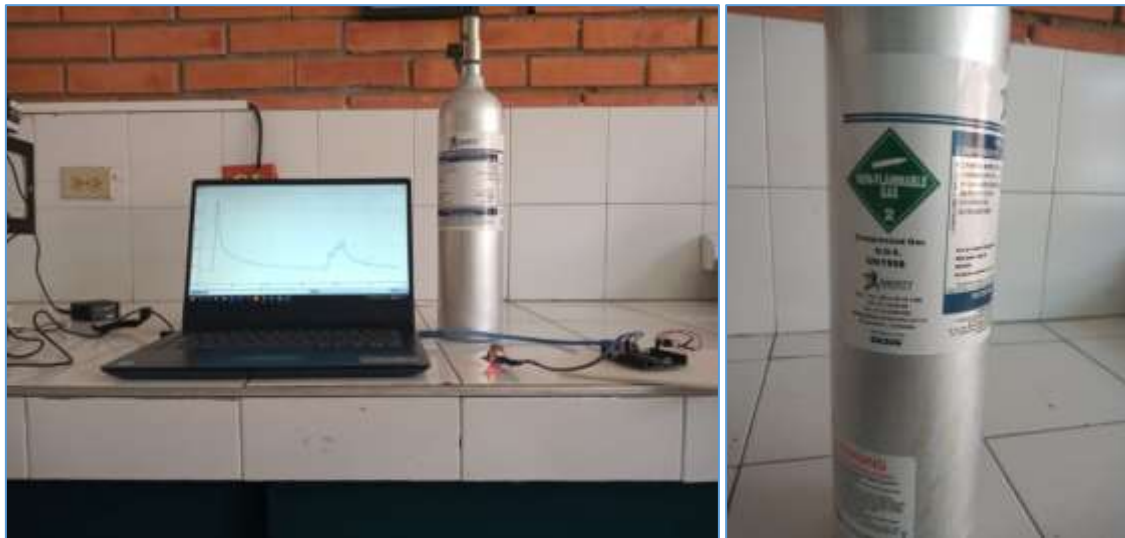
Figure 13. MQ4 sensor test, with mixed gases.
